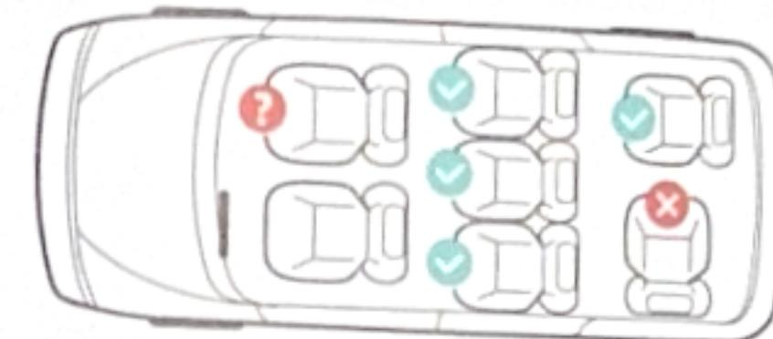
This ECRS is suitable for seat belt models equipped with the 3-point seat belt that has passed the ECE R16 requirement and is not suitable for models only equipped with 2-point seat belts.
